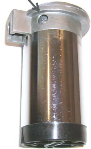
Air Intake Hole
